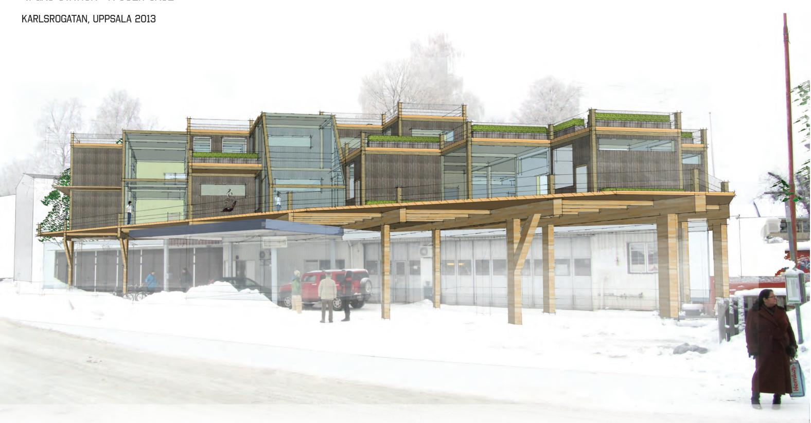
The modular concept has been applied to a project that is looking into reducing the demand for student accommodation while tackling the problem of wasted space in central locations. Here the modular basegrid is stilted on top of and around a disused gas station. In this example, we have changed the layout by retrofiting a two storey housing unit.
