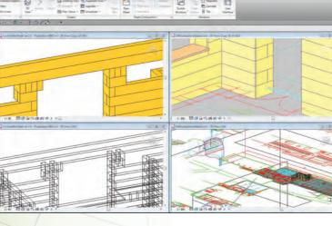
The structure is designed in cad where the 3D model information is integrated with the saw, where the structure is cut part by part produced with cnc-machinery.
